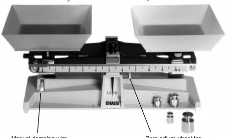
Manual damping wire loop for speedier weighings and teaching of damping principle.
